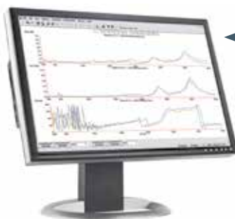
Bode Plot, showing overall vibration level, order 1 vibration and phase information
