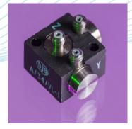
Lightweight triaxial vibration transducer compromising three Konic Shear® fully welded sensing inserts bonded orthogonally into a hard anodized aluminum housing.
