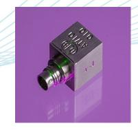
A lightweight miniature charge output triaxial vibration transducer with a single 4 pin connector, this is a unique design from DJB and comprises three charge output accelerometer piezo-electric elements mounted orthogonally within a titanium block. The use of the Konic Shear® independent sensing elements ensures a rugged and repeatable triaxial measurement under the most extreme conditions.
