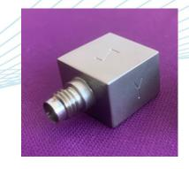
A lightweight general purpose PE charge output tri-axial vibration transducer comprising of three charge output Konic Shear® piezoelectric sensing elements mounted orthogonally within a titanium block with fully welded construction. The AT/04/TB is one of only 3 PE charge output single connector accelerometers in the world, all produced by DJB Instruments. This is possible due to the unique low noise four core cable supplied by DJB to reduce triboelectric noise.
