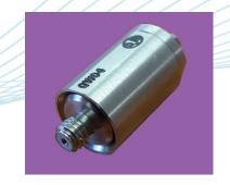
In-line charge to voltage converters provide users with the ability to use charge accelerometers with all their benefits of high temperature a robust build whilst using the built in IEPE signal conditioning power available in many off-the-shelf vibration controller/analysers and data acquisition front ends.
