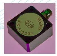
The AMB range of accelerometers are Biaxial MEMS (micro electro mechanical system) DC response voltage output devices for testing at low frequency vibration measurement from DC (0Hz) and above. They are Biaxial (measuring in 2 directions simultaneously) variable capacitance design. The AMB/50HR.40C has a 4 pin 1/4-28UNF side entry connector.
