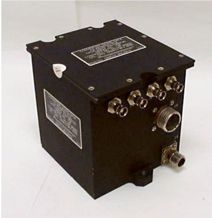
Systems & Electronics, Inc. (SEI) *Signal Data Converter (SDC), CV-4318/ASH-37* offers the capability of acquiring data from dual MIL-STD-1553 busses and has a real time clock. The data acquired from these busses and real time clock are transmitted to SEI's multiplatform *Structural Data Recording Set (SDRS), AN/ASH-37(v)* via RS-232. The SDRS is a multi aircraft data acquisition system. The unit presented in this technical data sheet is currently on the Navy's EA-6B aircraft.
